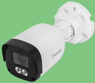
TC-C321N Spec:13/E/Y/2.8mm Analog Killer 1080p, 2.8mm, D-WDR, 3D-DNR, IR: 30m
